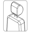
3 Rotate the brackets to an angle that will allow the brackets fit through the headrest posts.
